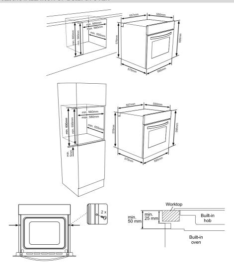
Insert the oven into the cabinet by pushing it If the oven is installed under a hob, the forward. Open the oven door and insert 2 screws distance between the worktop and the top in the holes located on the oven frame. While the panel of the oven must be minimum 50 mm product frame touches the wooden surface of and the distance between the worktop and cabinet, tighten the screws.
